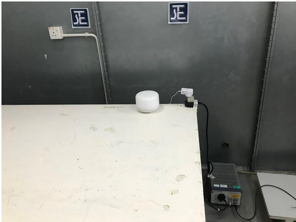
Measurement of Conducted Emission Test Set Up
