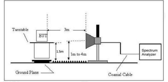
Frequency :9kHz-30MHz RBW=10KHz, VBW =30KHz Sweep time= Auto Trace = max hold Detector function = peak Frequency :30MHz-1GHz RBW=120KHz, VBW=300KHz Sweep time= Auto Trace = max hold Detector function = peak Frequency :Above 1GHz RBW=1MHz, VBW=3MHz(Peak), 10Hz(AV) Sweep time= Auto Trace = max hold QP Detector function = peak, AV
