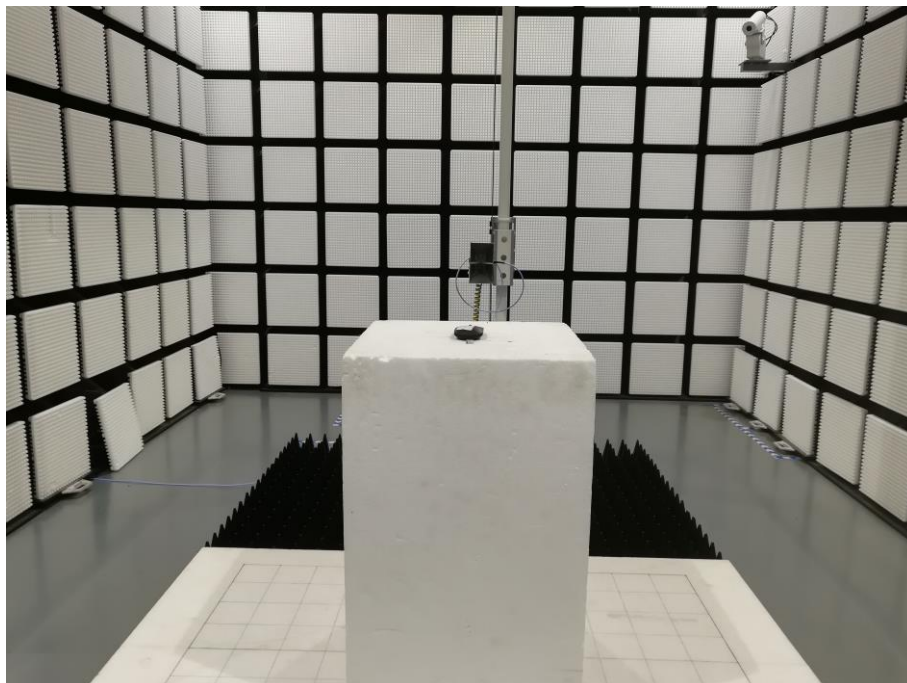
Fig. 3 Radiated emission setup photo(Above 1GHz)
