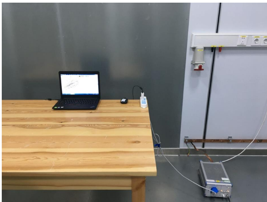
Fig. 4 Power line conducted emission setup photo
