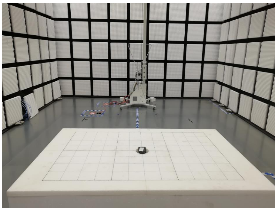
Fig. 2 Radiated emission setup photo(30MHz- 1GHz)
