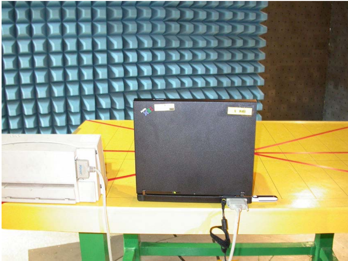
Photo 3: Radiated Emission Test set-up photo
