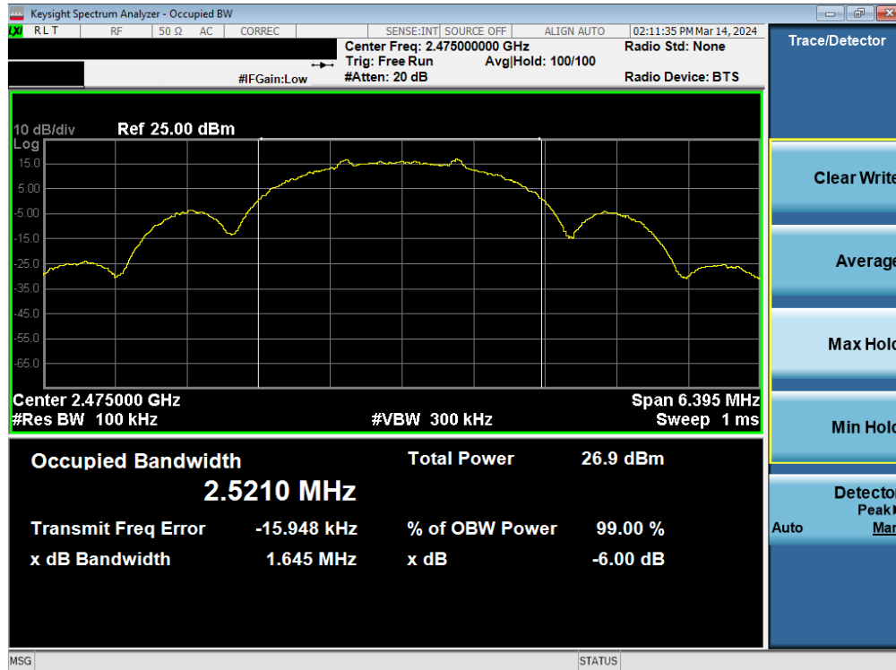
Plot 7-3. 6dB BW & 99% OBW Antenna 4a (802.15.4, Ch. 25)
