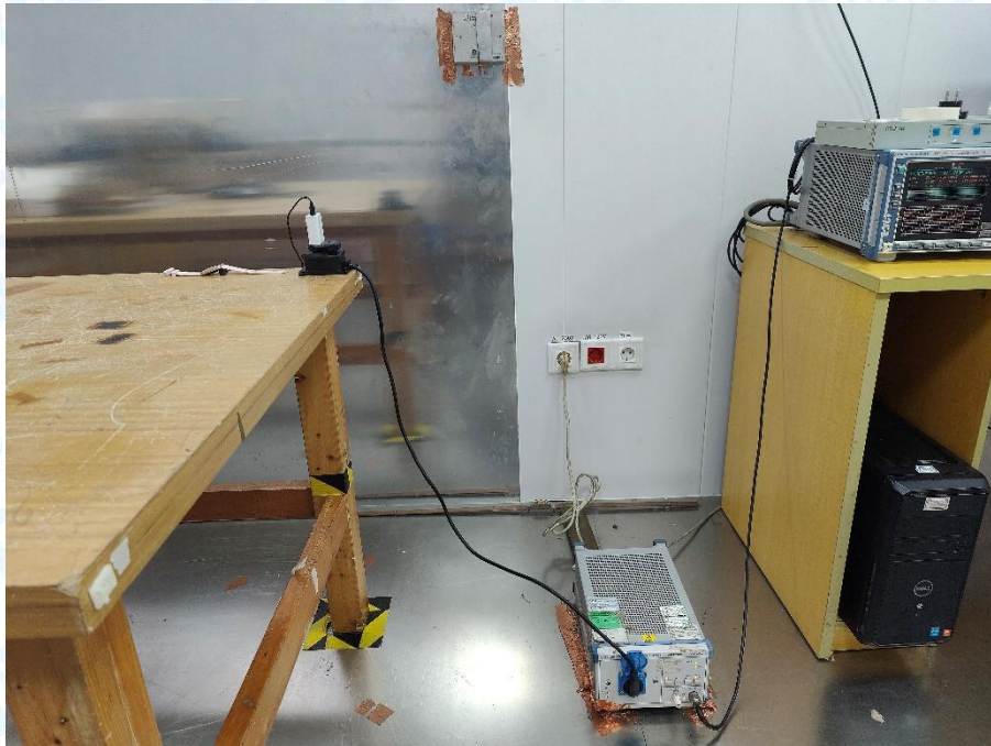
Photo of Setup for Radiated Emission (30MHz~1GHz)
