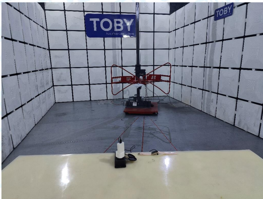
Photo of Setup for Radiated Emission (30MHz~1GHz)
