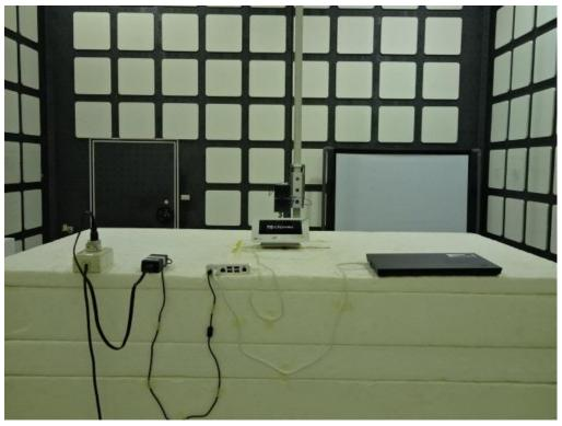
Radiated Emission Set up Photos (Front View)
