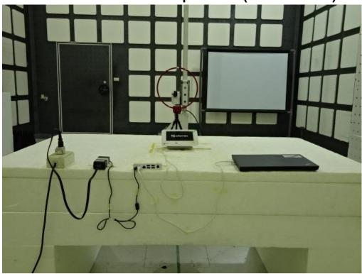
Radiated Emission Set up Photos (Below 1GHz)
