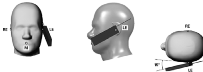
Figure 7.3 Front, Side and Top View of Ear/15° Tilt Position
