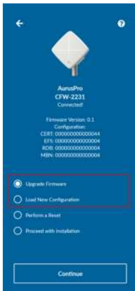
Figure 6 – Dashboard of Aurora Pro app when connected to the Outdoor CPE
