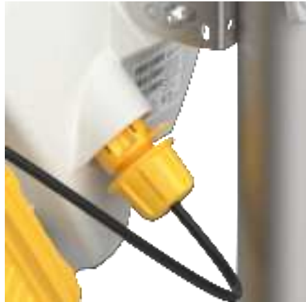
Figure 5 - Smart Installation Tool connected to PoE port of the Outdoor CPE
