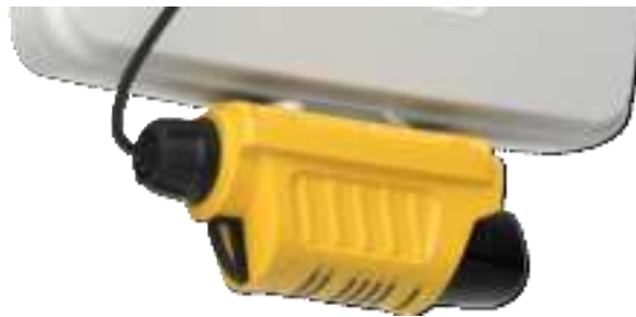
Figure 4 - Smart Installation Tool mounted on Outdoor CPE
