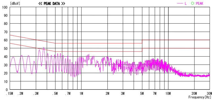
CHART: WITH FACTOR, Peak hold data. Data is uncorrected. CALCULATION: RESULT=READING+C.F(LISN LOSS+CABLE LOSS)
