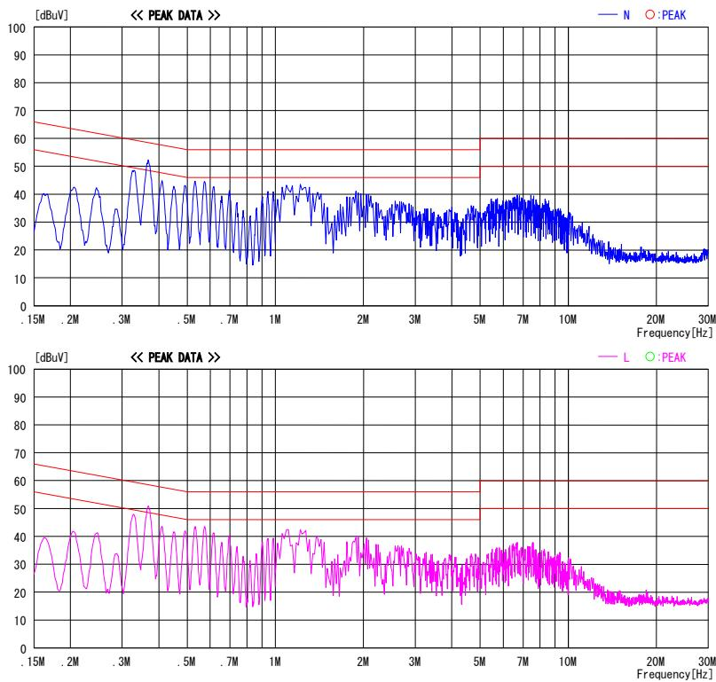
CHART: WITH FACTOR, Peak hold data. Data is uncorrected. CALCULATION: RESULT=READING+C.F(LISN LOSS+CABLE LOSS)
