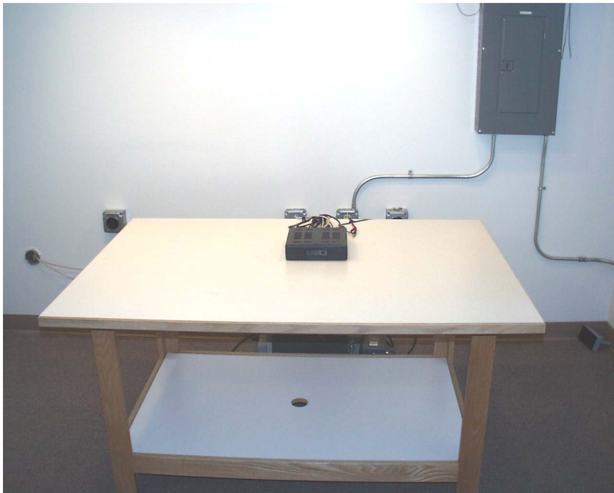
Front View Conducted Disturbance Worst Case Configuration
