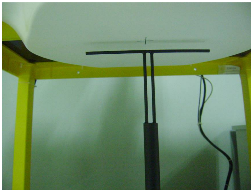
Fig 6.2 Setup Photo of Dipole Antenna
