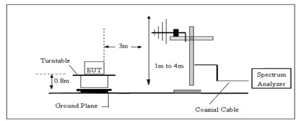
(B) Radiated Emission Test-Up Frequency Above 1GHz
