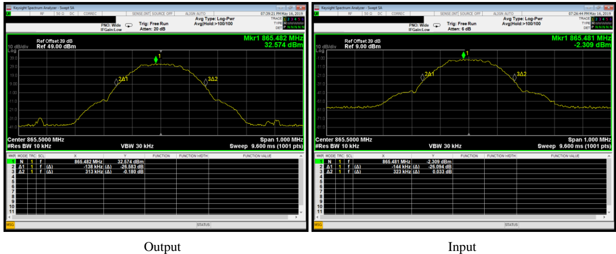
Plot 3.2.1: Input-versus-output signal comparison, MSK, Gaussian filter 0.3, data rate 270kbps, 0.5 dB below AGC threshold level
