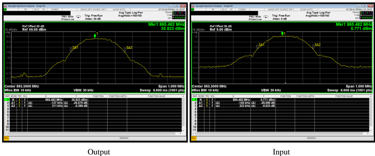
Plot 3.2.2: Input-versus-output signal comparison, MSK, Gaussian filter 0.3, data rate 270kbps, 3 dB above AGC threshold level
