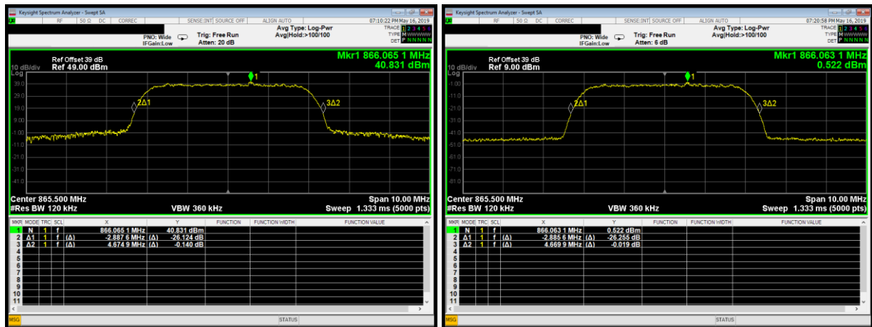
Plot 3.2.4: Input-versus-output signal comparison, AWGN 4.1MHz, 3 dB above AGC threshold level
