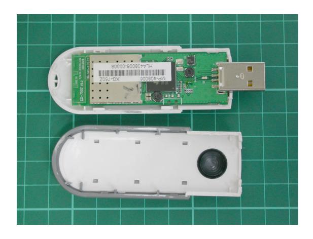
**Photo 2: Internal photo of EUT**
