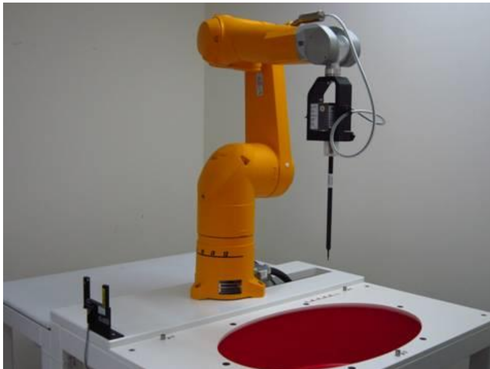
Fig.1 Photograph of the SAR measurement system
