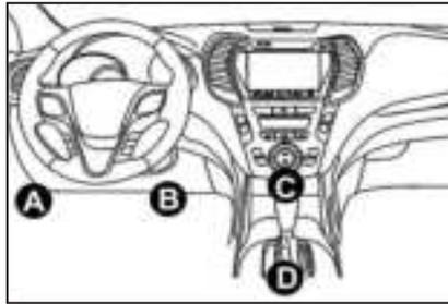
3. Plug the TOPDON ArtiDiag800 BT 2 Diagnostic MDCI Mini dongle into the vehicle's DLC socket.
