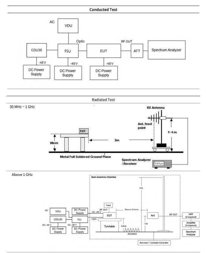
\* EUT position is adopted by placement of floor-standing refer to section 5.5.2.3.2 of ANSI C63.26-2015
