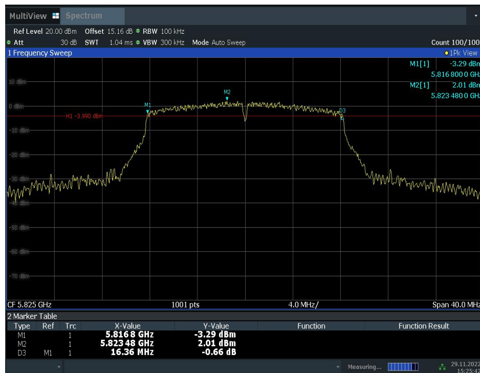
Fig. 2 Occupied 6dB Bandwidth (802.11a, Ch 157)
