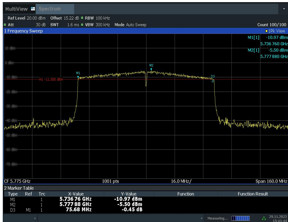
Fig. 8 Occupied 6dB Bandwidth (802.11ac-VHT40, Ch 159)
