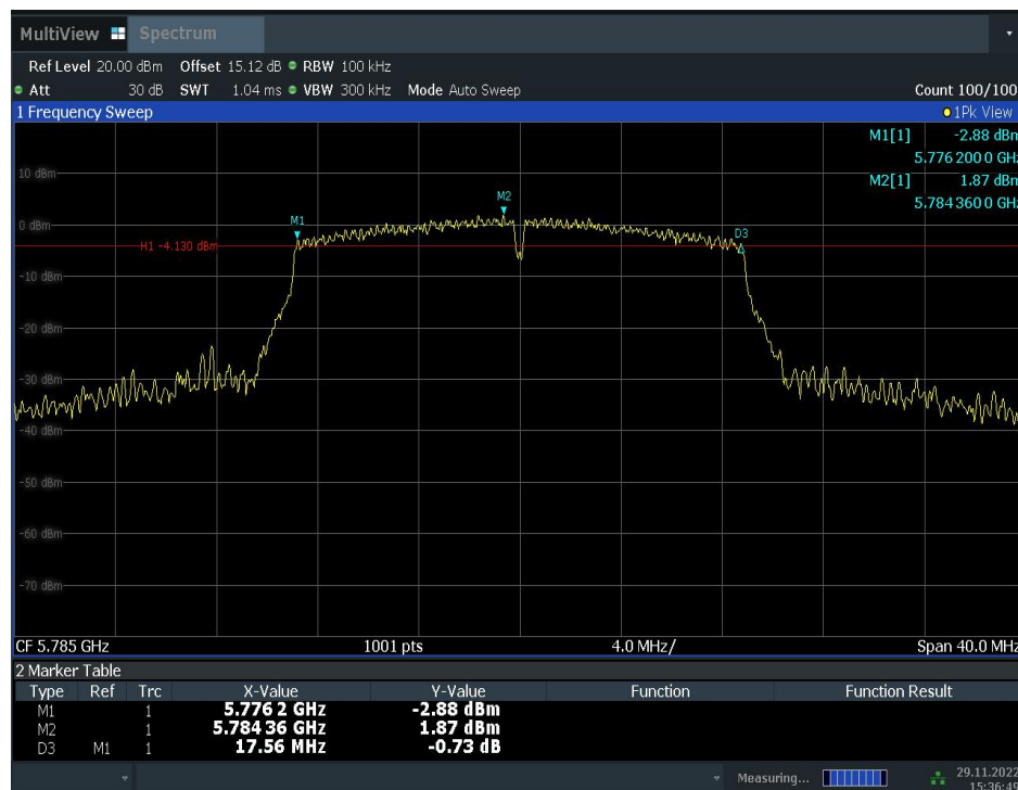
Fig. 4 Occupied 6dB Bandwidth (802.11ac-VHT20, Ch 149)
