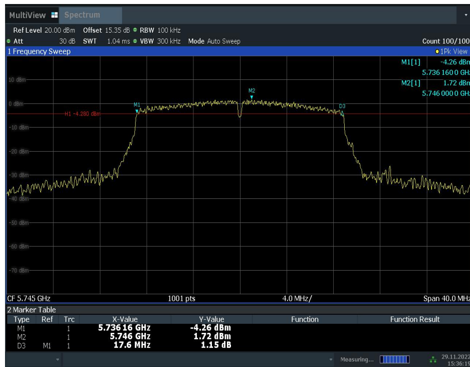
Fig. 4 Occupied 6dB Bandwidth (802.11ac-VHT20, Ch 149)
