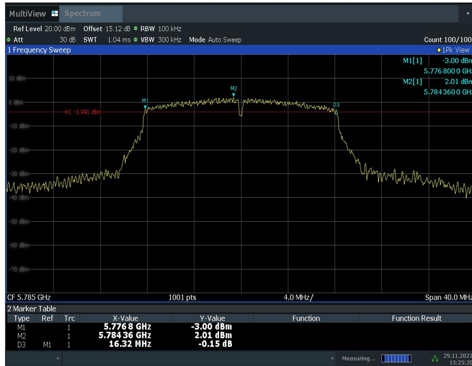
Fig. 1 Occupied 6dB Bandwidth (802.11a, Ch 149)
