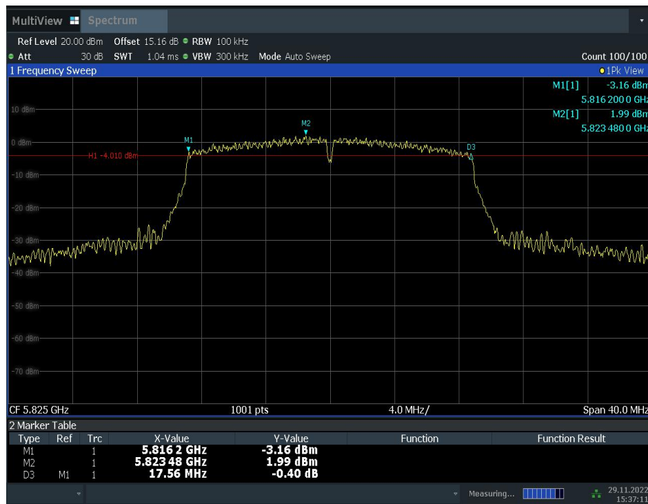
Fig. 6 Occupied 6dB Bandwidth (802.11ac-VHT20, Ch 165)
