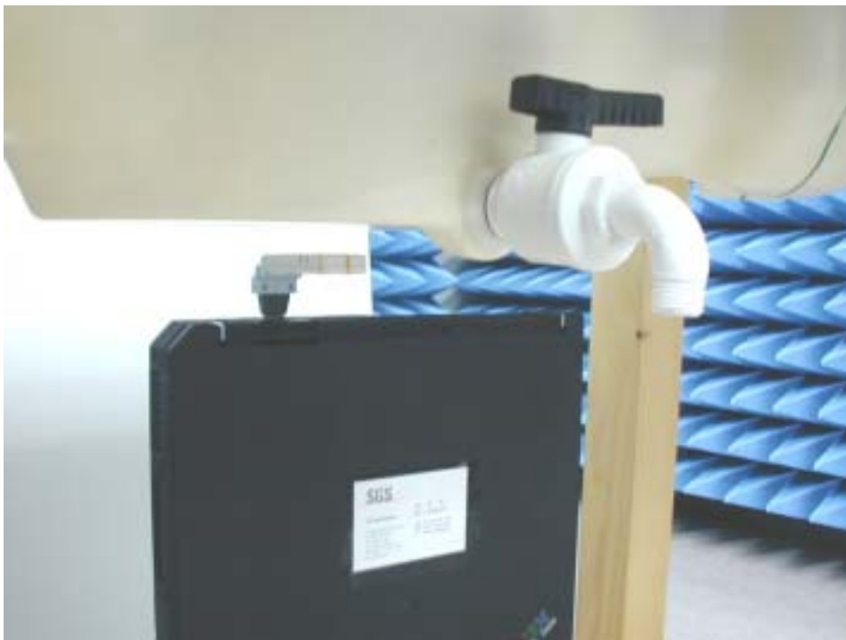
Fig.2 Photograph of the edge of the PC at 90° and at a distance of 1.5 cm from the base of the phantom and the antenna is in horizontal direction.
