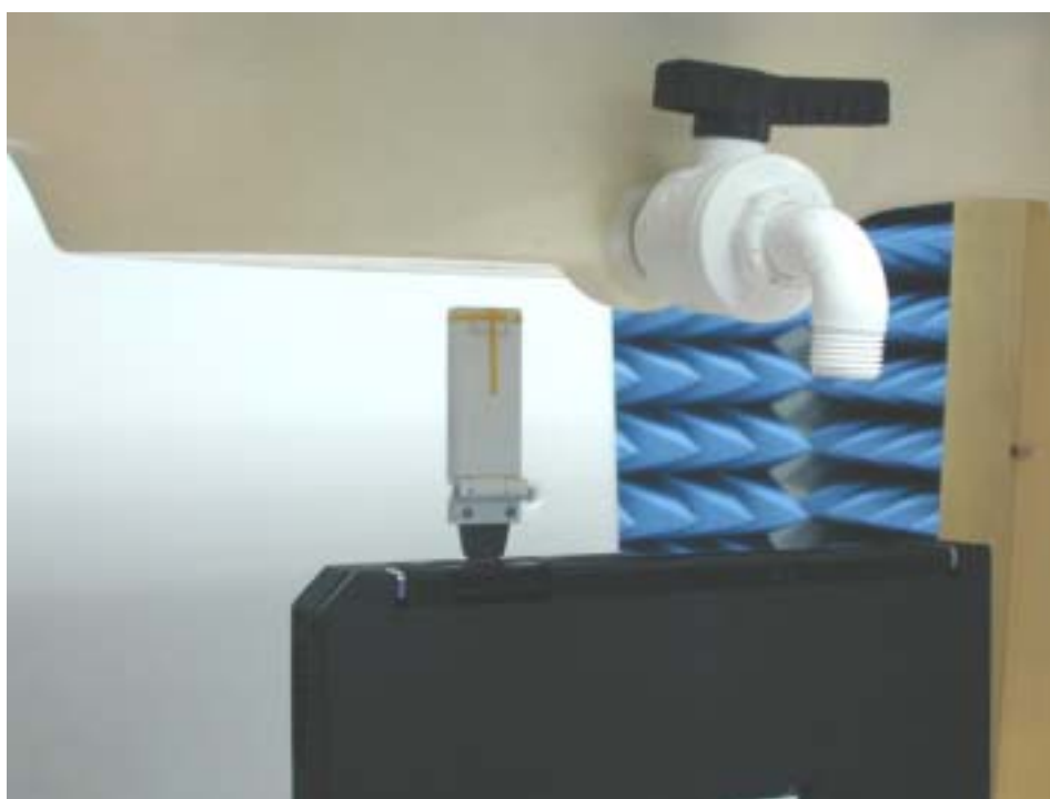
Fig.4 Photograph of the edge of the PC at 90° and at a distance of 1.5 cm from the base of the phantom and the antenna tip upward.
