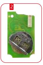
Take the battery out and replace new one Note: The battery type is 2032 with 3V, ensure the positive and negative of battery is correct.
