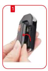
Break open the back side plastic cover to open the remote
