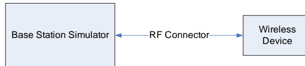
Figure 9-3 Power Measurement Setup
