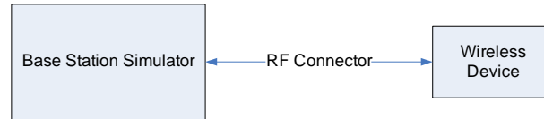
Figure 9-5 Power Measurement Setup – NR Online
