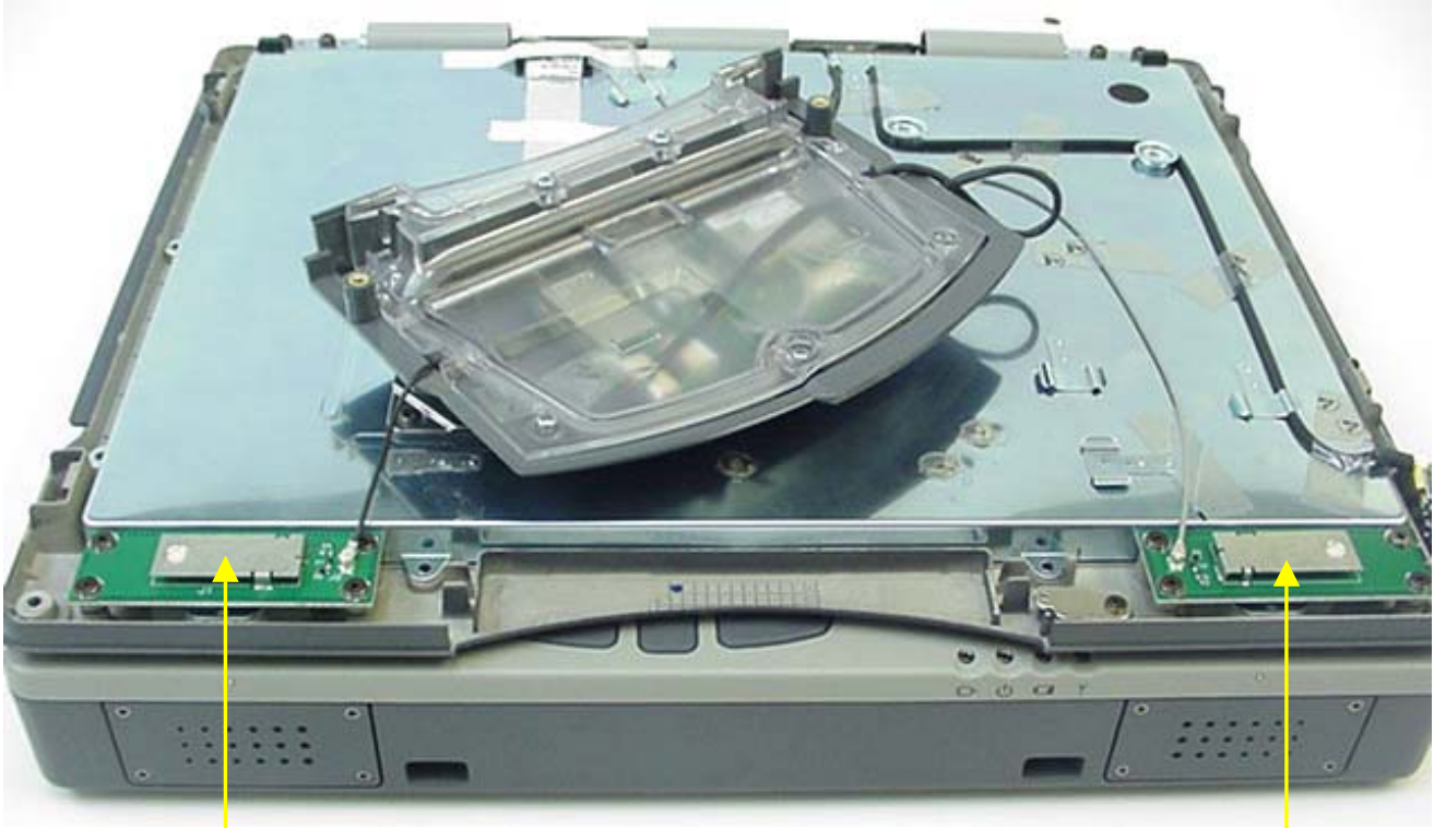
Bluetooth Surface-Mount Antenna (Upper Left Side Rear Edge of LCD Display)
