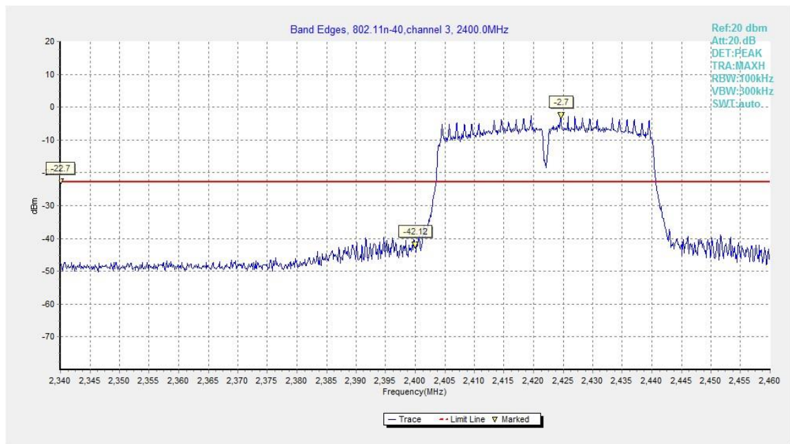
Fig.A.5.7 Band Edges (802.11n-HT40, Ch 3)
