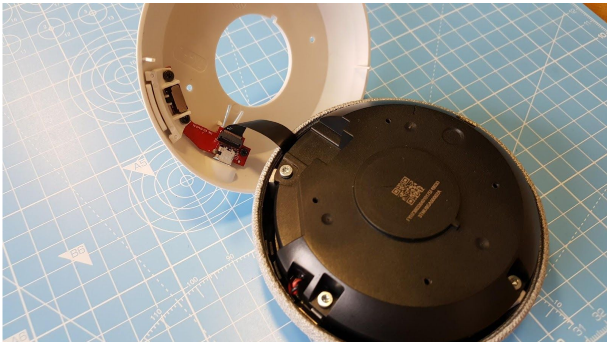
Speaker and Ribbon Cable to USB Port Close-up
