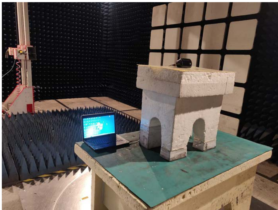
Spurious Emission Test Setup (Above 1GHz)
