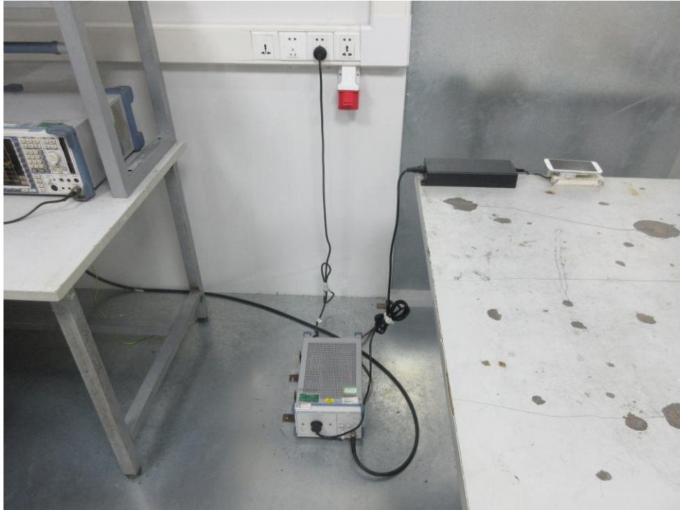
Photo of Power Line Conducted Emission Test
