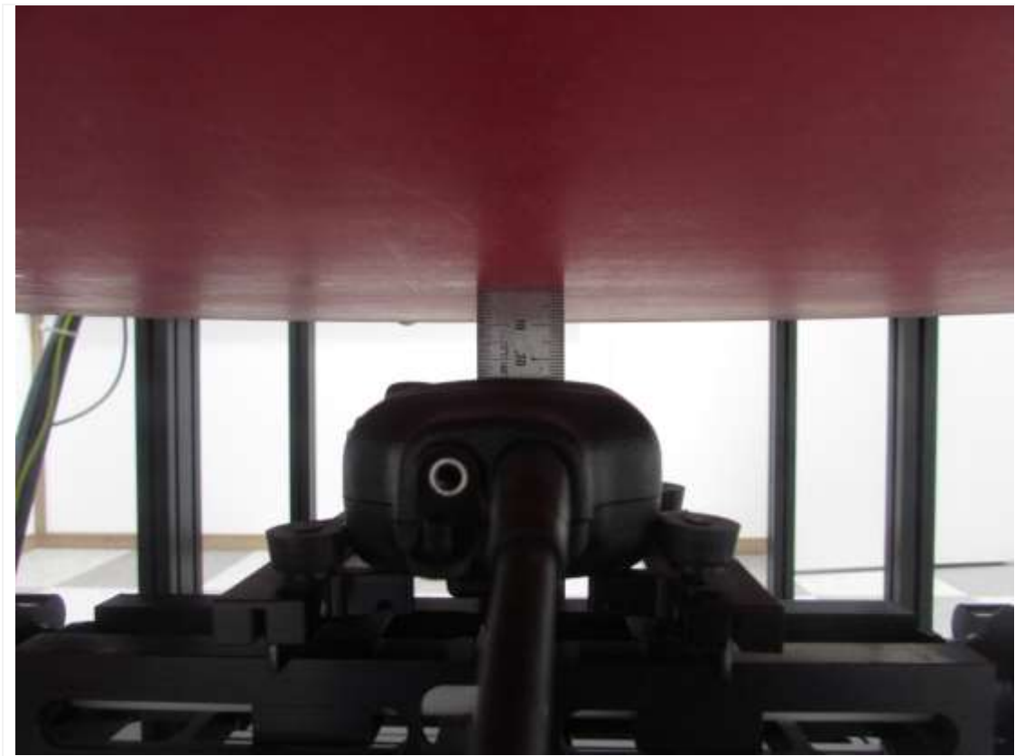
Distance of 25 mm from the EUT
