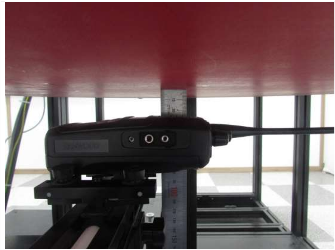
Distance of 25 mm from the EUT
