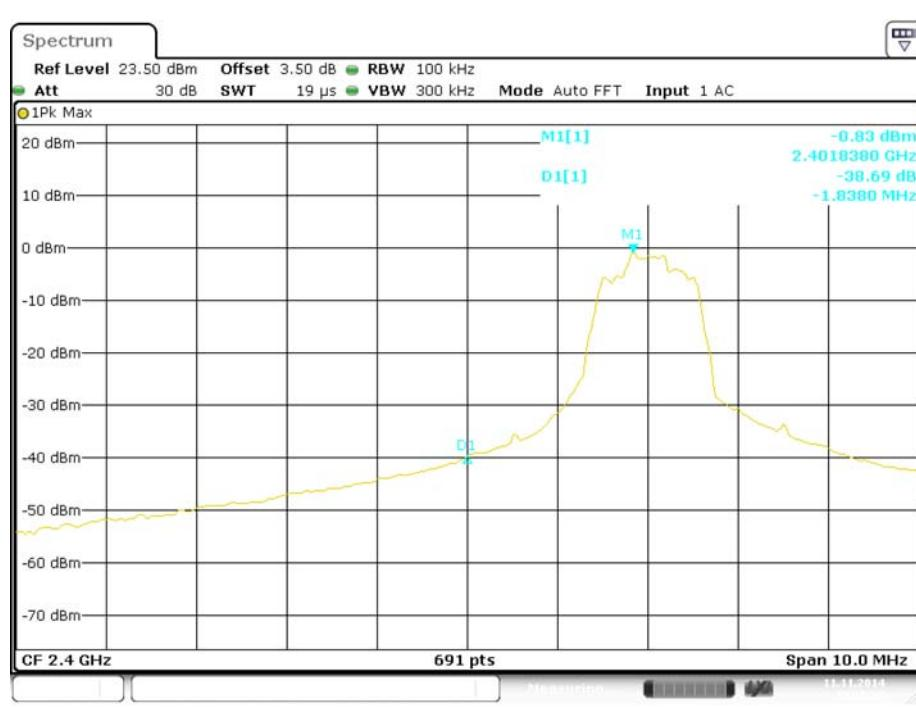
**EDR ( $\pi/4$ -DQPSK): Band Edge-Right Side**
