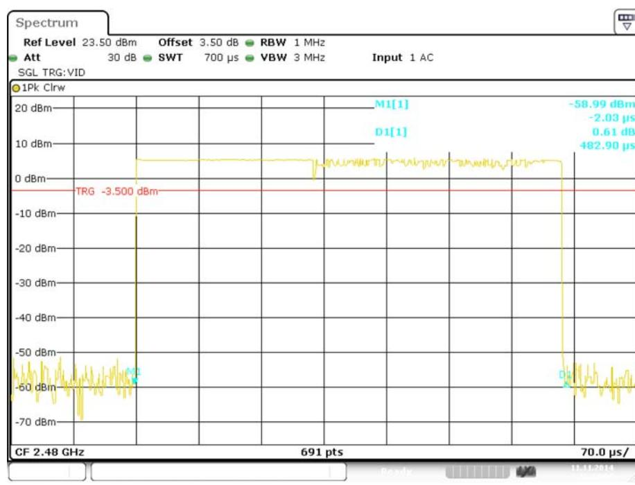
**Pulse time, Low Channel, DH3**
