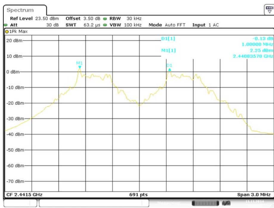
**BDR (GFSK): High Channel**
