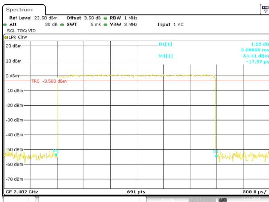
**Pulse time, Middle Channel, DH5**
