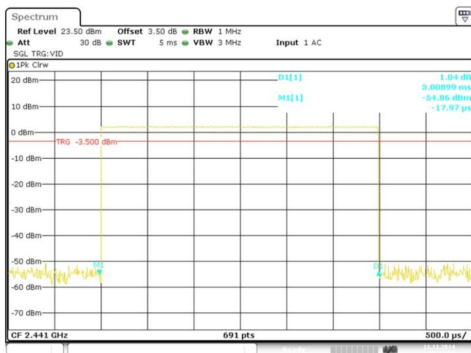
**Pulse time, High Channel, DH5**
