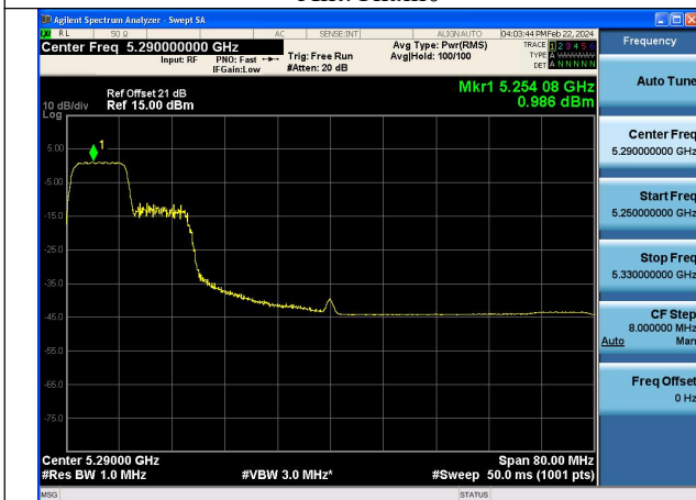
Mode:802.11ax HE80 Tone:106T Frequency:5290MHz Ant:Chain0
