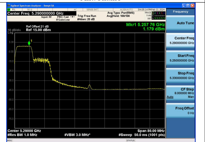
Mode:802.11ax HE80 Tone:106T Frequency:5290MHz Ant:Chain1
