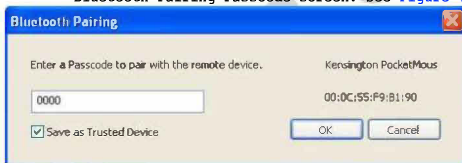
Figure 4-2. Entering Bluetooth Pairing Passcode
