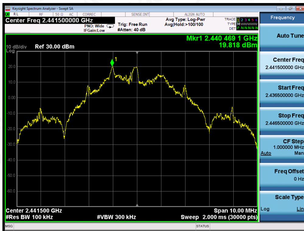
TEST PLOT OF OUT OF BAND EMISSIONS OF GFSK MODULATION IN MIDDLE CHANNEL
