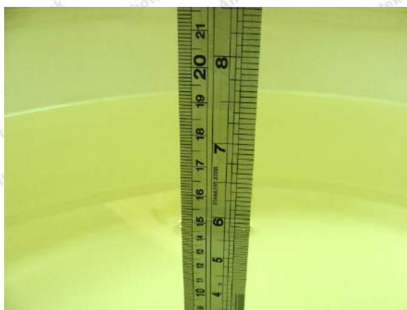
Photo of Liquid Height for Body SAR
