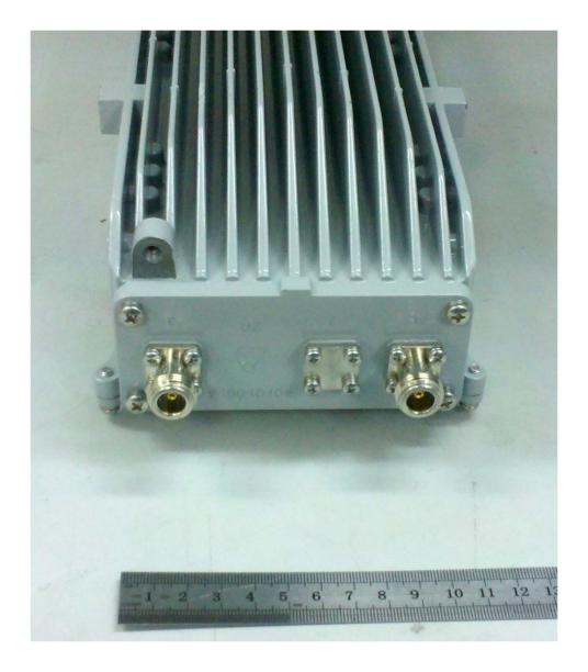
Photograph No.2 "Synergy 2000 2.5 GHz (B41)" base station top panel view
