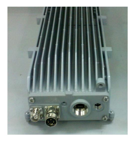
Photograph No.4 "Synergy 2000 2.5 GHz (B41)" base station bottom panel view
