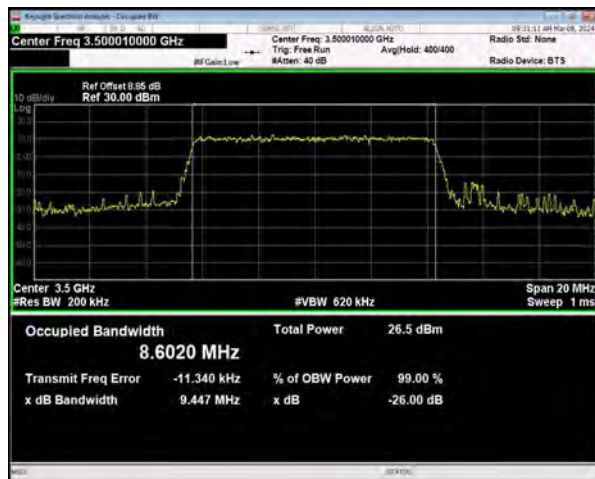
n77(3450-3550) SCS=30kHz CP_QPSK BW=10MHz Channel=633334 RB=24@0
