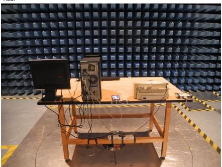
AC Conducted Emission Test Setup Setup- EUT+ Battery+ PC +LCD monitor Front
