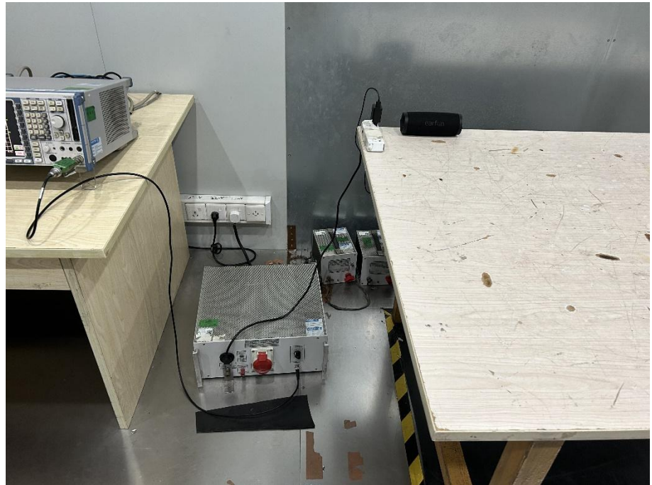
Conducted Emission Test Setup
