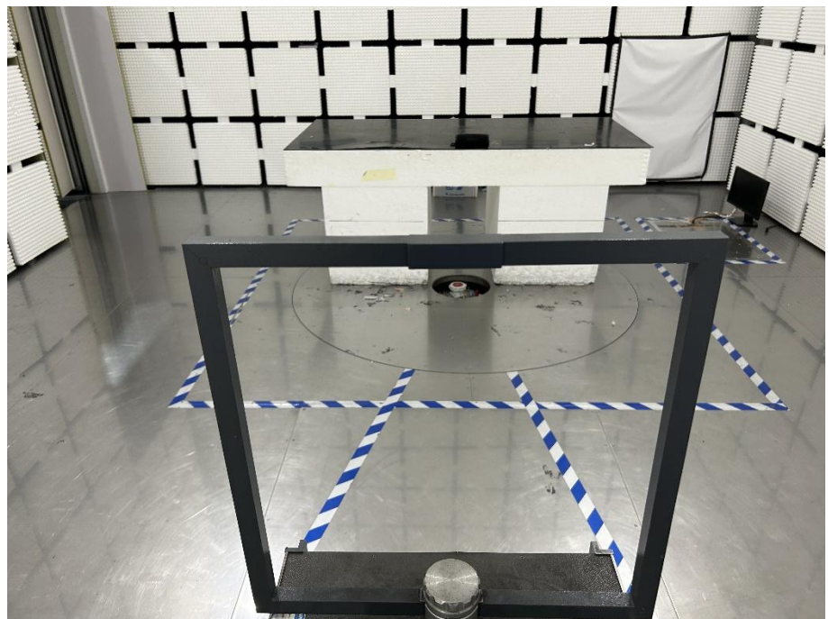
Radiation Emission Test Setup (Below 30MHz)
