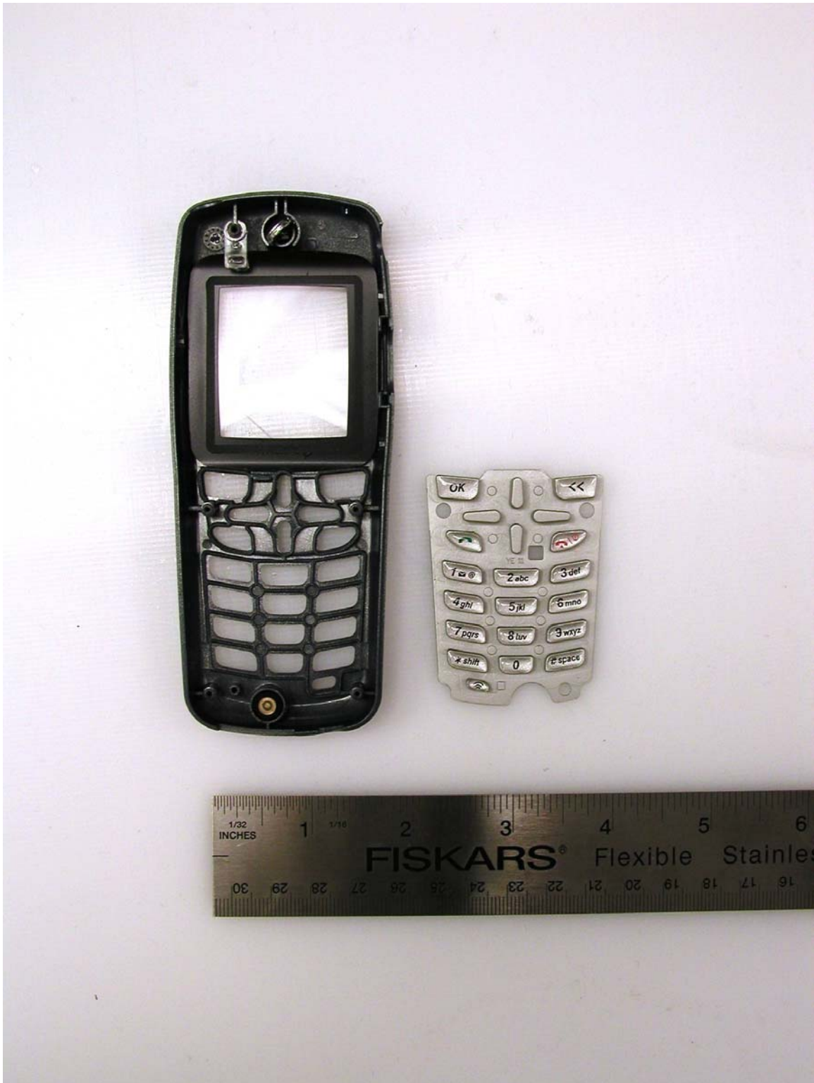
Figure 2-11 Front housing with keypad removed
