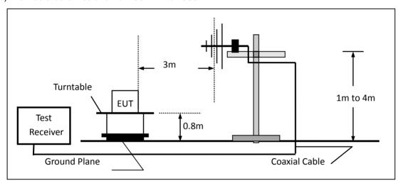
(c) For radiated emissions above 1000MHz
