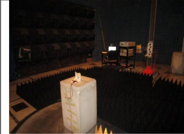
**4-18 GHz Radiated Emissions RX mode (TX mode has pedestal at 150cm)**
