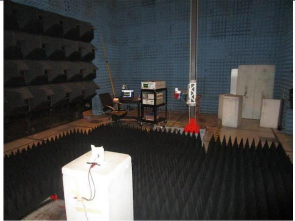
**18-25 GHz Radiated Emissions RX mode (TX mode has pedestal at 150cm)**
