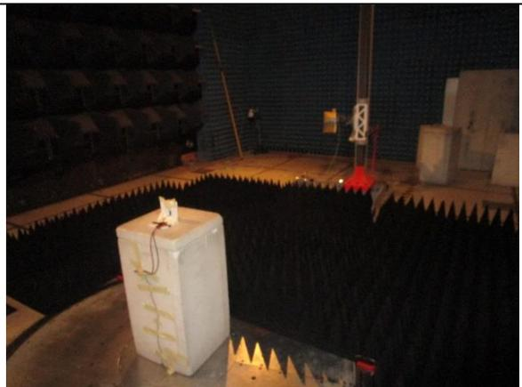
**1-4 GHz Radiated Emissions RX mode (TX Mode has pedestal at 150cm)**
