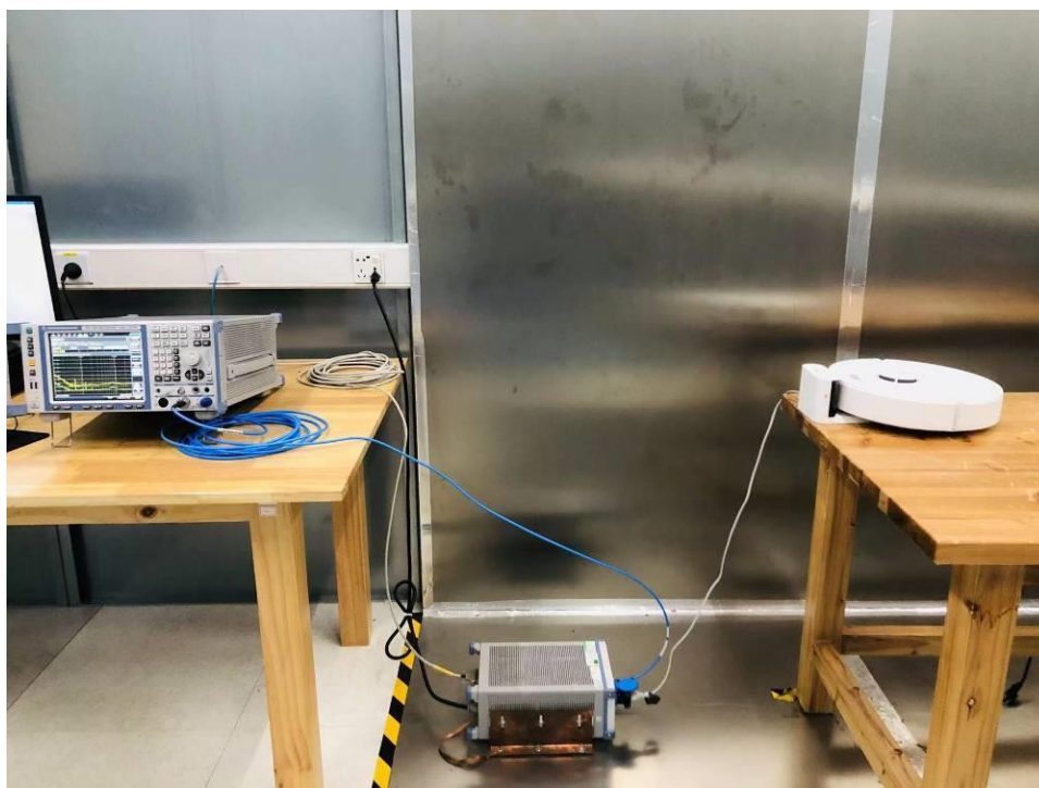
Photograph 3: Set-up photo for Conducted Emission
