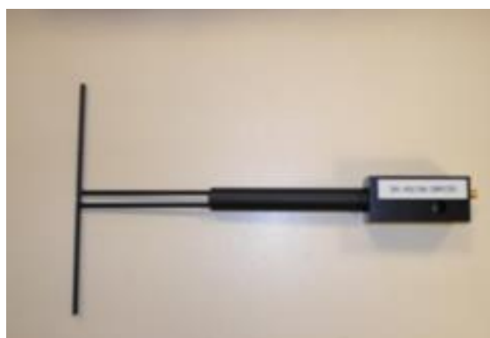
Figure 1 – MVG COMOSAR Validation Dipole
