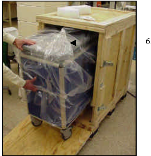
Figure 3: Removing Conversion Station and Backing Down Ramp
