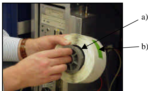
Figure 18: Installing Plastic Core Inserts on Ends of D1 Roll
