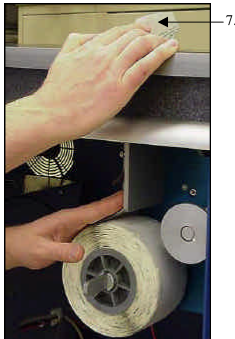
Figure 20: Threading the Leader Up Through Tag Feed Area
