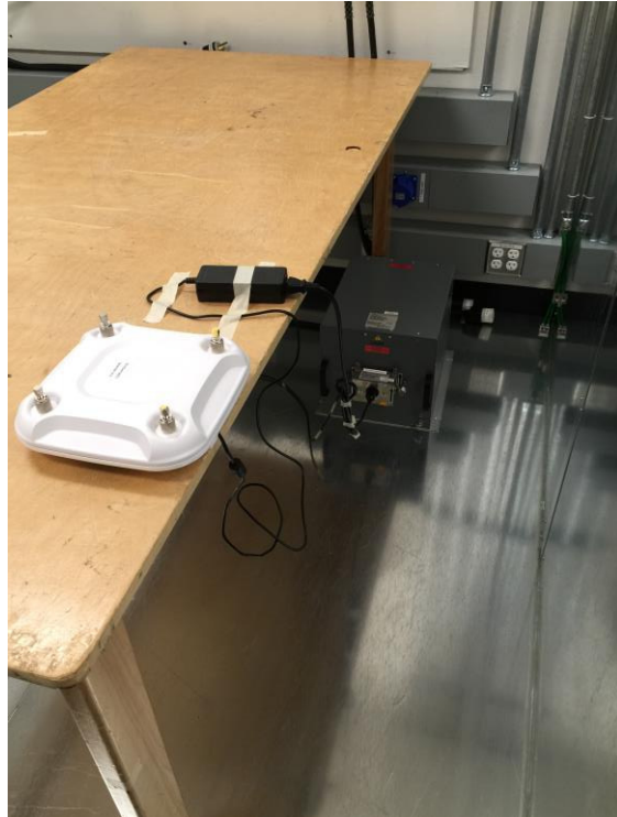
AIR-CAP3702P-B-K9 AC Conducted Emissions setup photo
