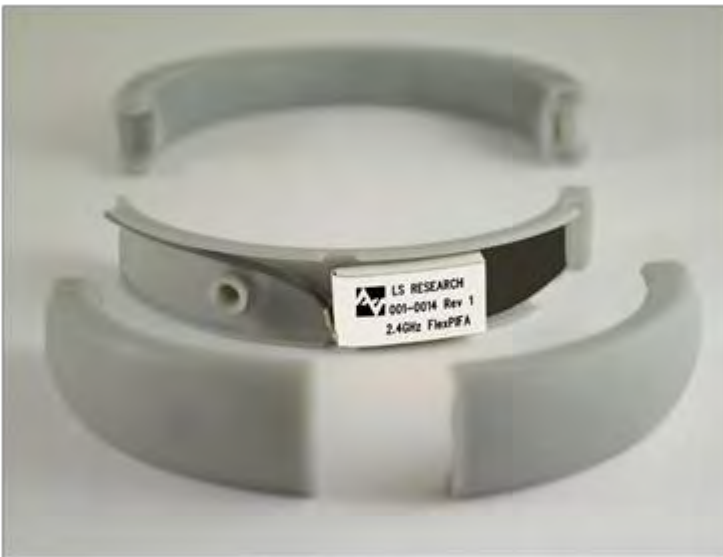
Figure 40: FlexPIFA integrated into bracelet
