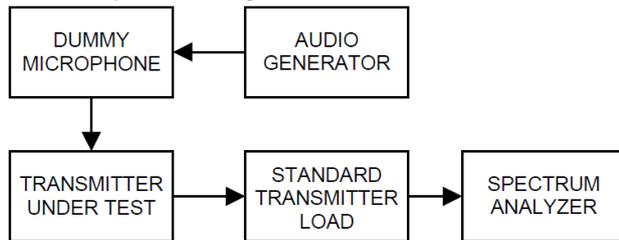
Test setup for Digital:
