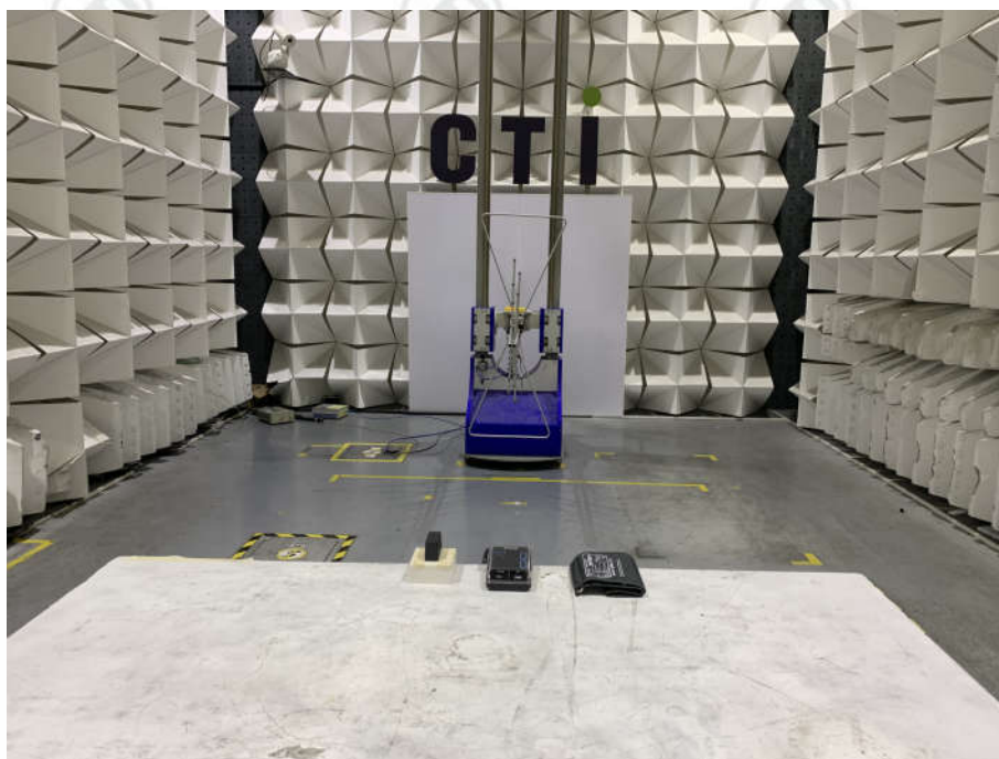
Radiated spurious emission Test Setup-1(Below 1GHz)
