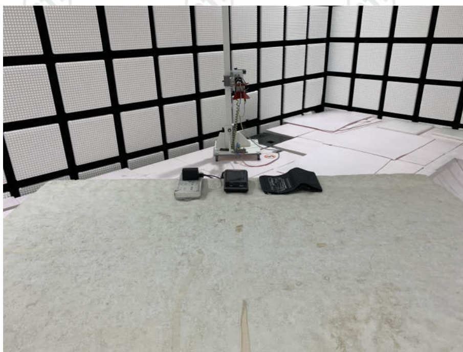
Radiated spurious emission Test Setup-2(Above 1GHz)
