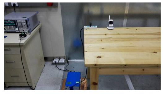
RADIATED EMISSION BELOW 1GHZ TEST SETUP
