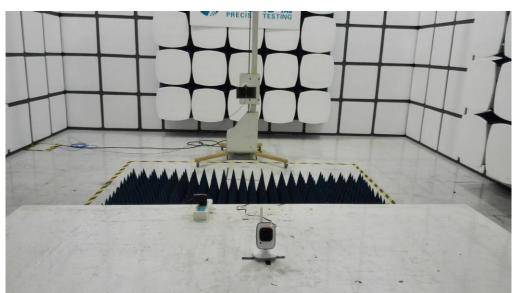
RADIATED EMISSION ABOVE 1GHZ TEST SETUP
