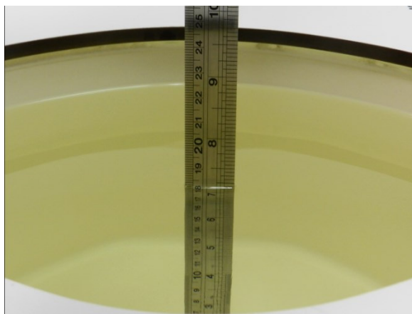
Fig 10.2 Photo of Liquid Height for Body SAR
