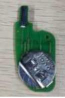
2, take the battery out and replace new one (Notes:the battery type is 2032 with 3 voltage,ensure the positive and negative of battery is correct)
